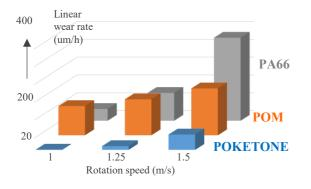
[Rotation speed 0.07m/s, Block load 15MPa]
