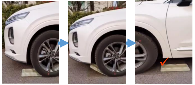
[POKETONE molded part of food tray No crack or brittle fracture after vehicle load]
