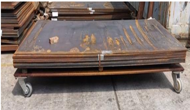
▲ PK Caster 3.2MT load test
